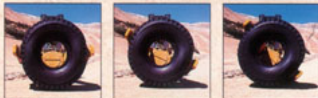
Only IMT TireHands provide up to 390° of body rotation.
